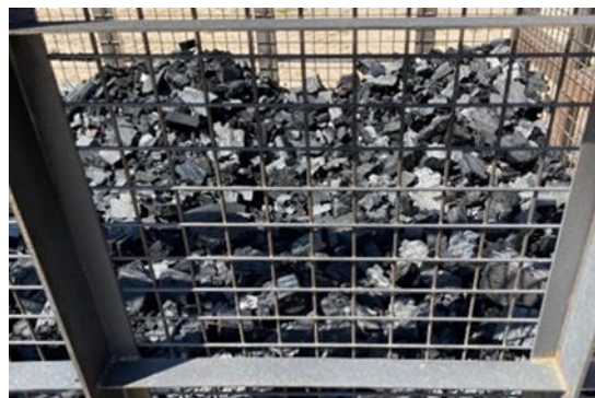
Following system run, bio-char, discovered, as a by-product of wood pallets placed in cage.
