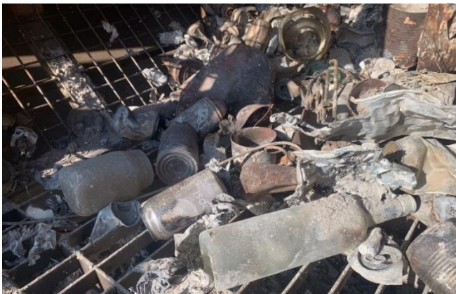
Picture to Left – close up shot of items left in the cage following emission test run. Note decals/color on aluminium cans not visible, but aluminium is still in place. Glass bottles/jars still in place. Fully recyclable. August 2021
