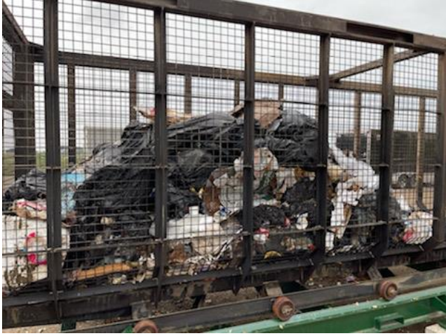
Above A load of Municipal Solid Waste (MSW) loaded in cage prior to cage being placed in the gasifier unit. August 2021
